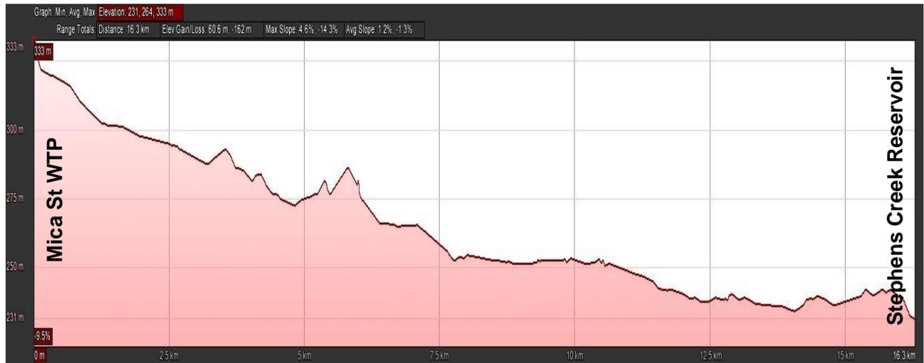
**Figure 3-3: Long-section profile of Stephens Creek Reservoir to Mica St WTP**
