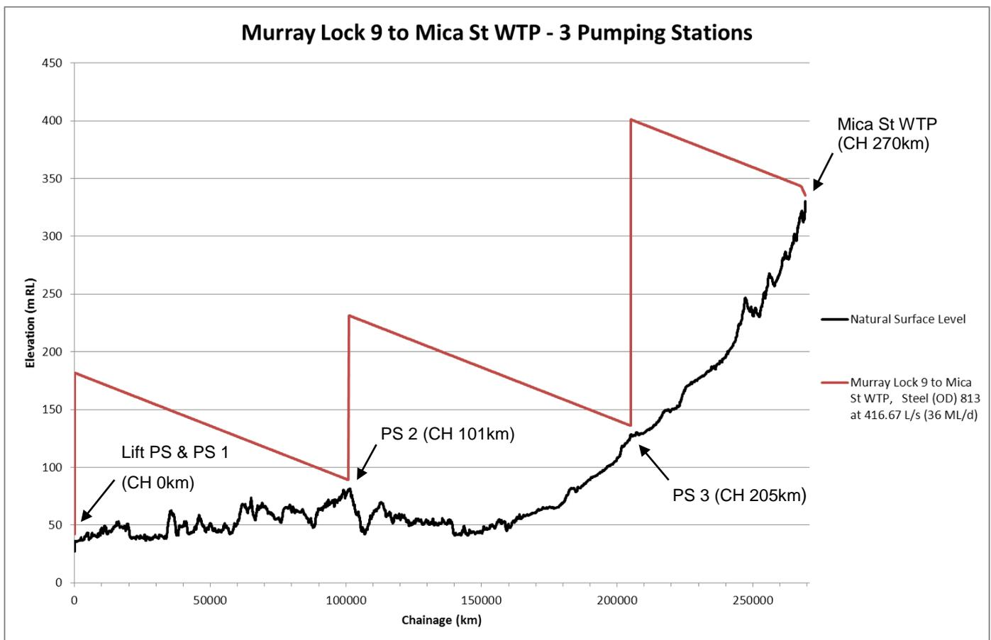
Figure 3-1: HGL for OD 813 x 8mm MSCL pipeline & three (3) transfer pumping stations
