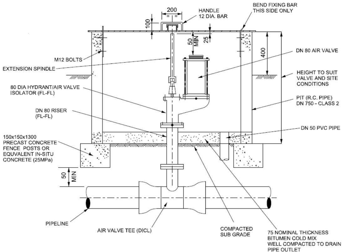
**Figure 3-2: Typical automatic on-line air release valve arrangement**
