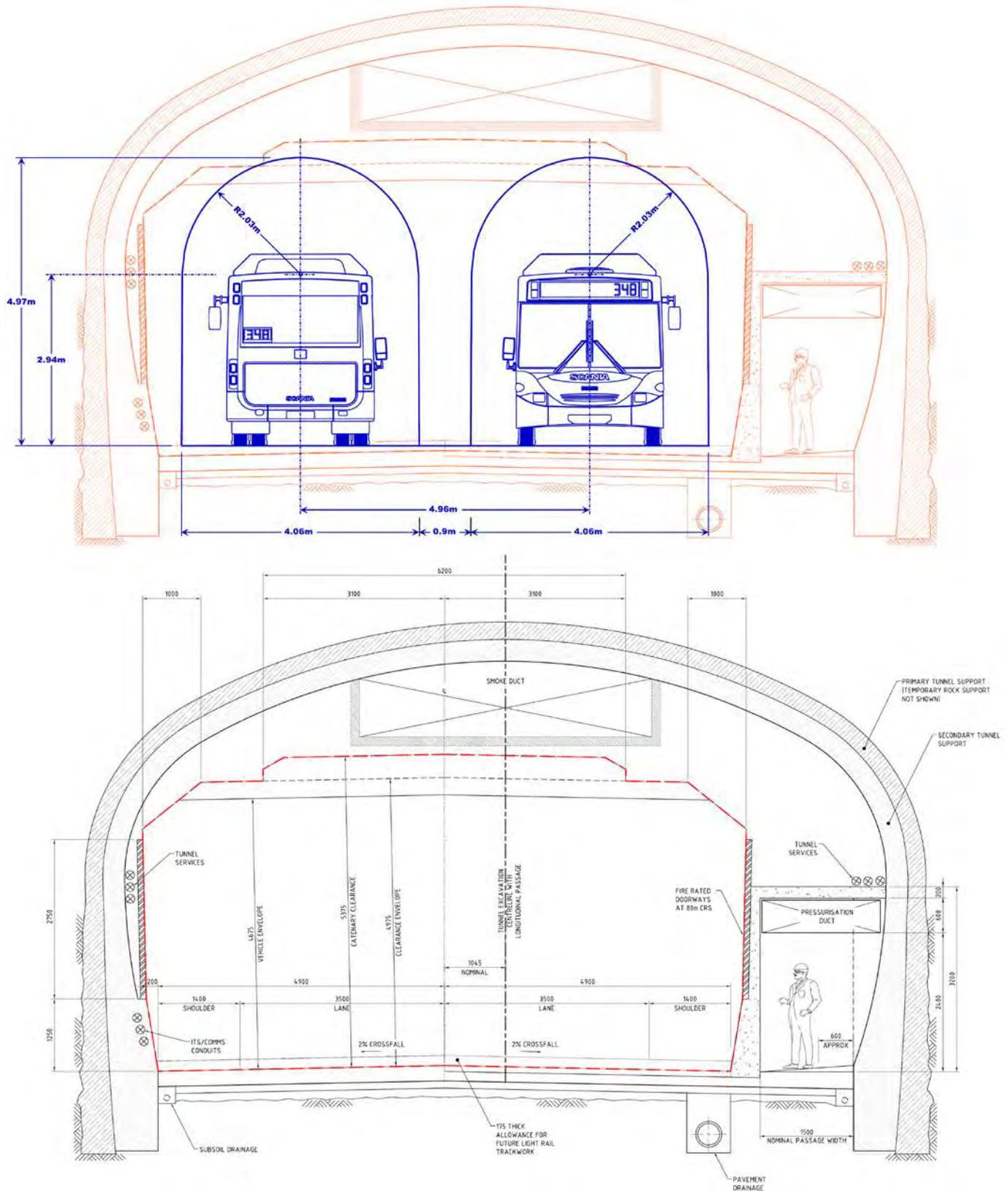
Figure 18: Comparison of Wynyard Tram Tunnel and Brisbane Busway Tunnel Sections
