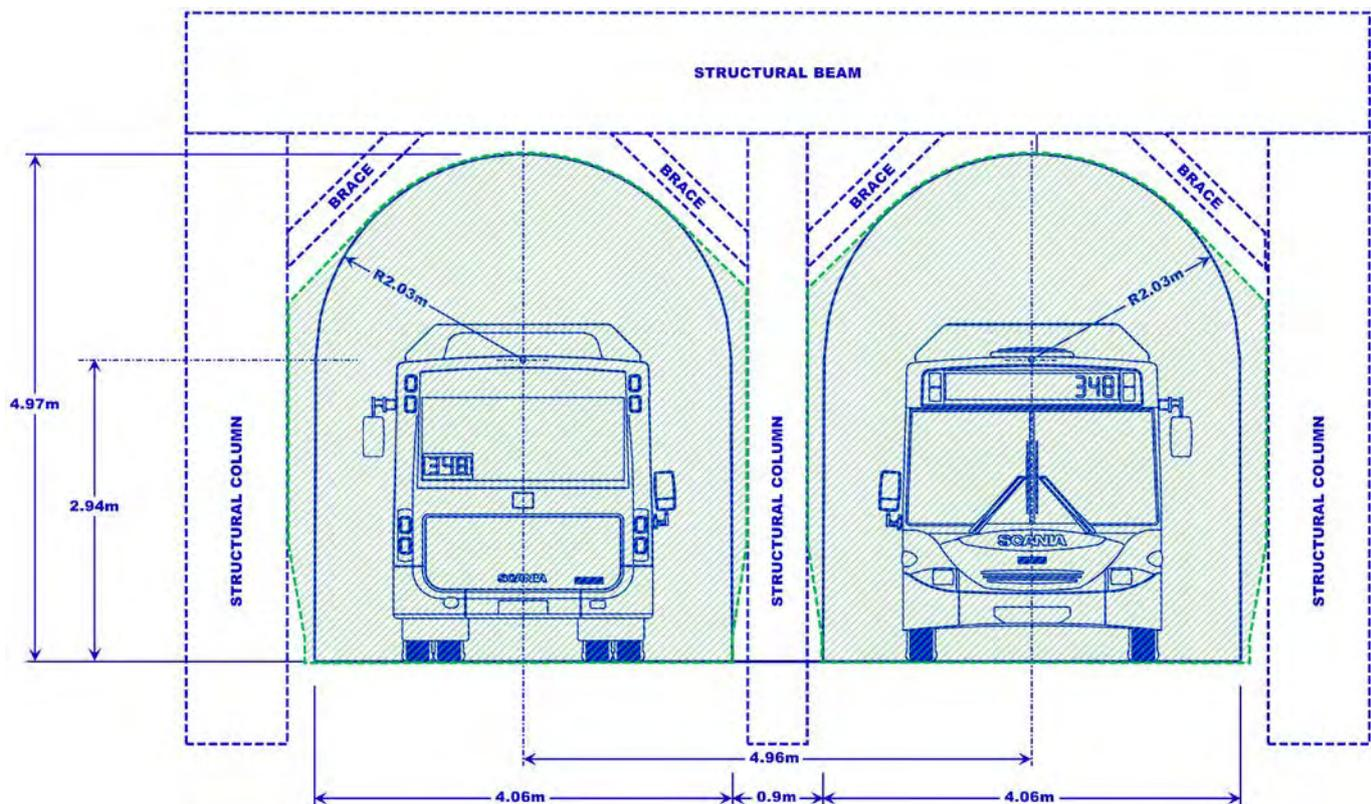
Figure 19: Potential Section Widening of Wynyard Tram Tunnels
