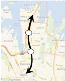
This concept includes an underground bus only tunnel system linking from the southern end of the Harbour Bridge to a location adjacent to Town Hall Station. The section from the Harbour Bridge to Wynyard Station coincides with existing tunnels that were built with the construction of the Sydney Harbour Bridge and carried two way tram traffic from 1932 to 1958.
