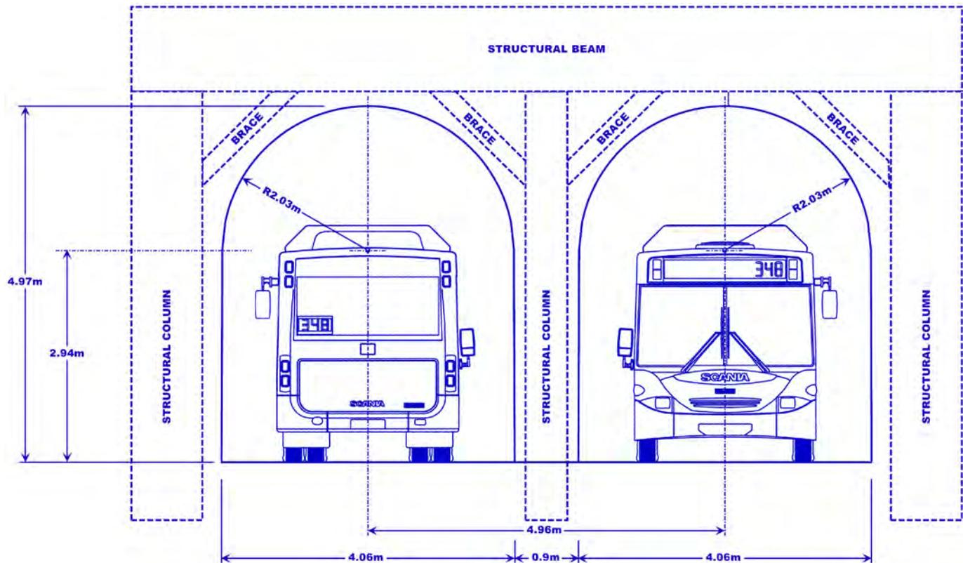
Figure 17: Wynyard Tram Tunnel As-Constructed Section
