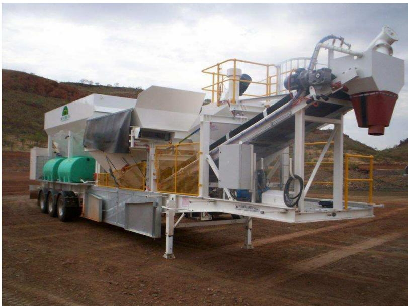
*JHG Modular Mobile Concrete Mixing Plant*
