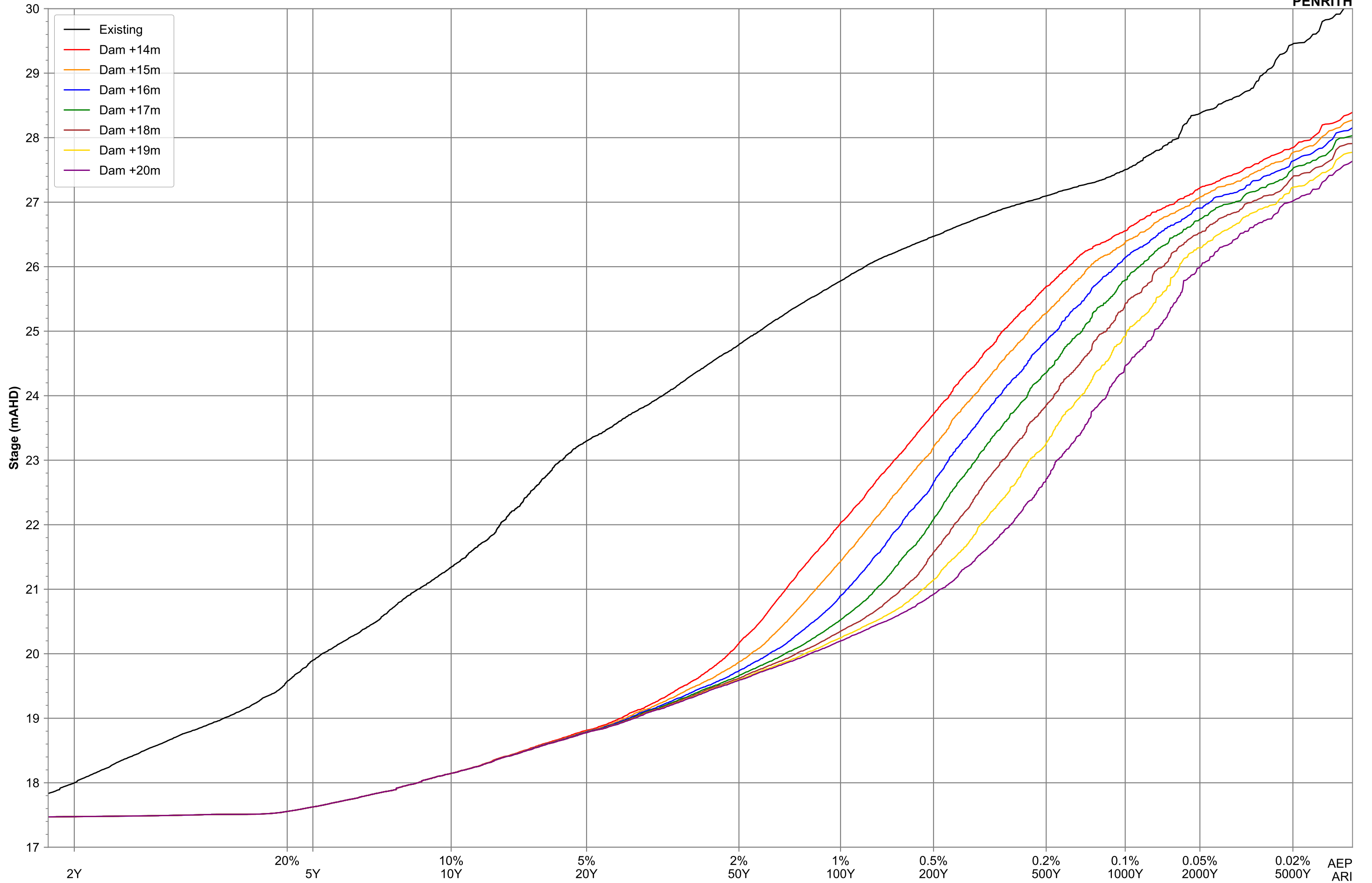
FIGURE A2 STAGE FREQUENCY CURVE DAM RAISING - NO CLIMATE CHANGE PENRITH
