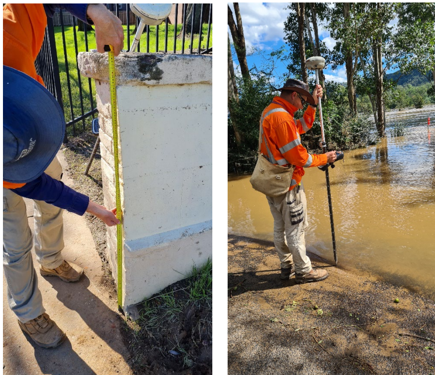
Figure 41: Surveying March 2021 flood levels to update flood models
