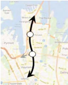
This concept includes an underground bus only tunnel system linking from the southern end of the Harbour Bridge to a location adjacent to Town Hall Station. The section from the Harbour Bridge to Wynyard Station coincides with existing tunnels that were built with the construction of the Sydney Harbour Bridge and carried two way tram traffic from 1932 to 1958.
