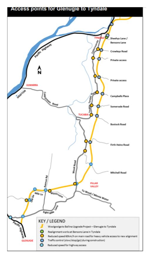
Figure 9 Gelnugie to Tyndale construction works alignment
